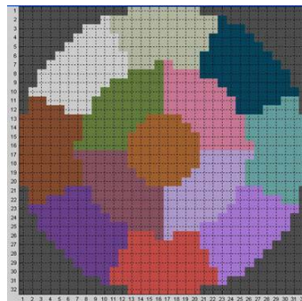
Figure 2. Typical 13-zone division of circular flow section derived from pixel grid
